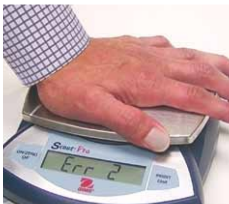
Mechanical and software overload protection
