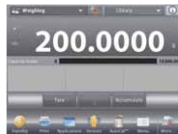
High resolution, 5.7" color TFT display
